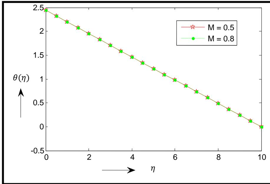
Fig. 10. Graph between dimensionless variable  $\eta$  and heat transfer of fluid  $\theta(\eta)$ ; this graph shows that the variation magnetic parameter  $M$  at constant embedding parameter  $p = 0.8$  and other parameter  $k = 0.5$ ,  $Pr = 0.7$ ,  $Gr = 0.5$ .
