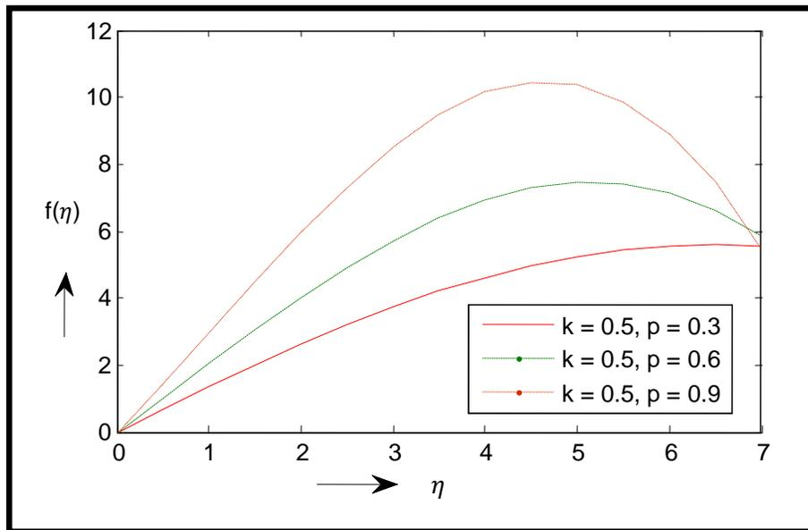
Fig. 1. Graph between dimensionless variable  $\eta$  and velocity of fluid  $f(\eta)$ ; this graph shows that the variation of embedding parameter  $p$  at constant value of  $Pr = 0.7$ ,  $Gr = 0.5$  and  $M = 0.1$ .
