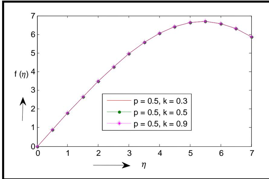
Fig. 2. Graph between dimensionless variable  $\eta$  and velocity of fluid  $f(\eta)$ ; this graph shows that the variation parameter  $k$  at constant value of  $Pr = 0.7$ ,  $Gr = 0.5$  and  $M = 0.1$ .
