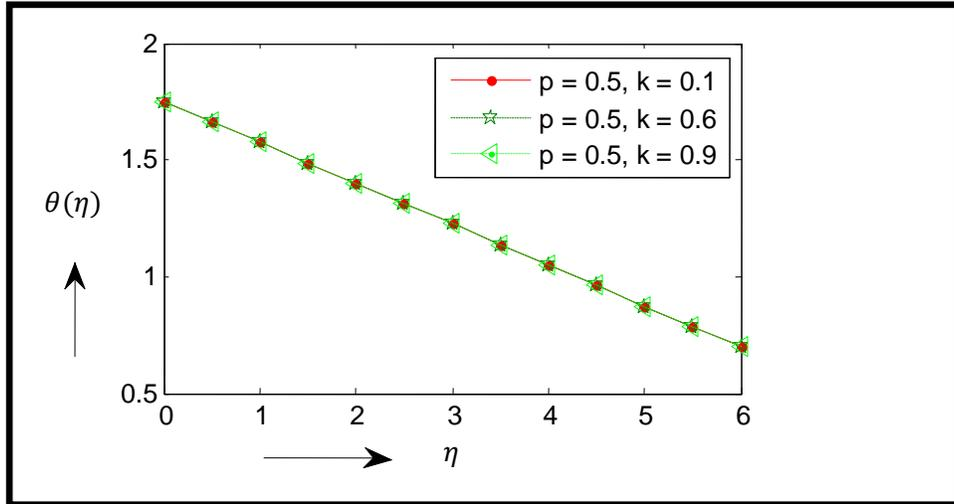
Fig. 4. Graph between dimensionless variable  $\eta$  and velocity of fluid  $\theta(\eta)$ ; this graph shows that the variation parameter  $k$  at constant value of  $Pr = 0.7$ ,  $Gr = 0.5$  and  $M = 0.1$ .
