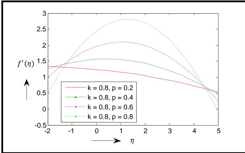
Fig. 6. Graph between dimensionless variable  $\eta$  and radial velocity of fluid  $f'(\eta)$ ; this graph shows that the variation of embedding parameter  $p$  at constant value of  $Pr = 0.7$ ,  $Gr = 0.5$  and  $M = 0.1$ .
