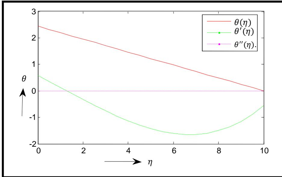
Fig. 8. Graph between dimensionless variable  $\eta$  and  $\theta(\eta), \theta'(\eta)$  &  $\theta''(\eta)$ ; this graph shows that the variation of derivative of  $\theta$  at constant embedding parameter  $p = 0.8$  and other constant parameter  $k = 0.5$ ,  $Pr = 0.7$ ,  $Gr = 0.5$  and  $M = 0.1$ .
