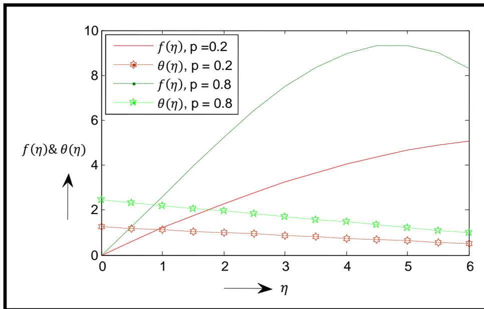
Fig. 5. Graph between dimensionless variable  $\eta$  and velocity of fluid  $f(\eta), \theta(\eta)$ ; this graph shows that the variation of embedding parameter  $p$  at constant value of  $Pr = 0.7$ ,  $Gr = 0.5$  and  $M = 0.1$ .
