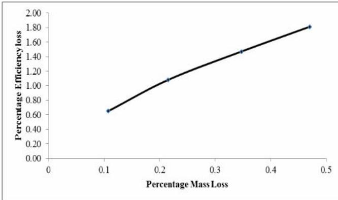
Figure 7. Percentage efficiency loss versus percentage mass loss of turbine
