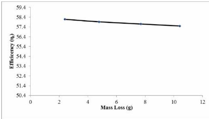
Figure 6. Turbine efficiency versus bucket mass loss
