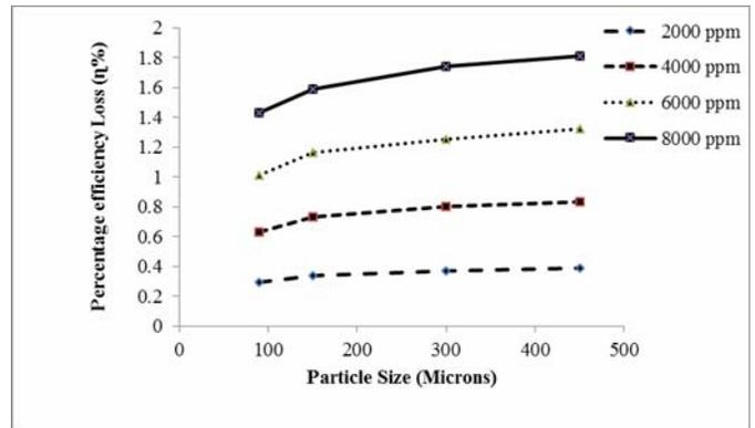
Figure 4. Percentage efficiency loss versus silt size
