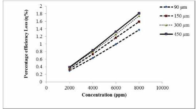
Figure 3. Percentage efficiency loss versus silt concentration
