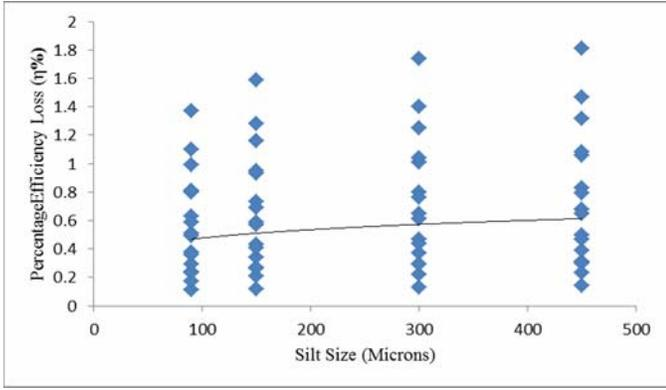
Fig.9. Plot of percentage efficiency loss versus silt size
