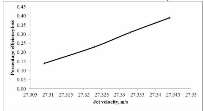
Figure 8. Percentage efficiency loss versus jet velocity
