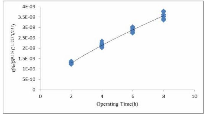
Figure 12. Plot of  $\frac{\eta_{\%}}{S^{0.166} C^{1.1223} V^{2.413}}$  versus operating time
