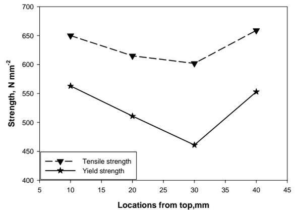
Fig.3.b. Strength at different location @ SAW
