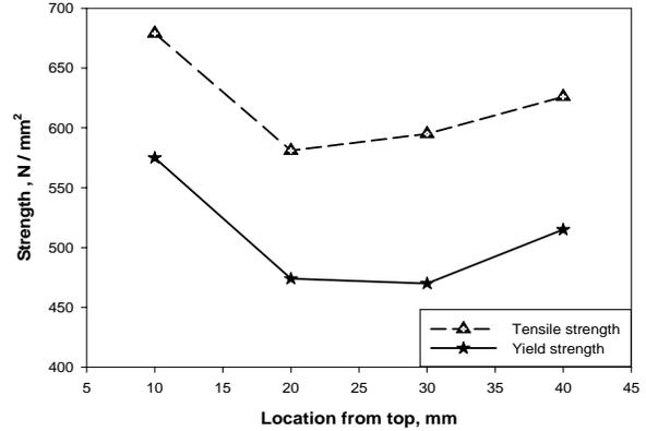
Fig.3.a. Strength at different location @ SMAW
