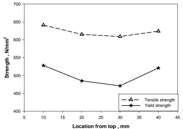
Fig.3.c. Strength at different location @ FCAW
