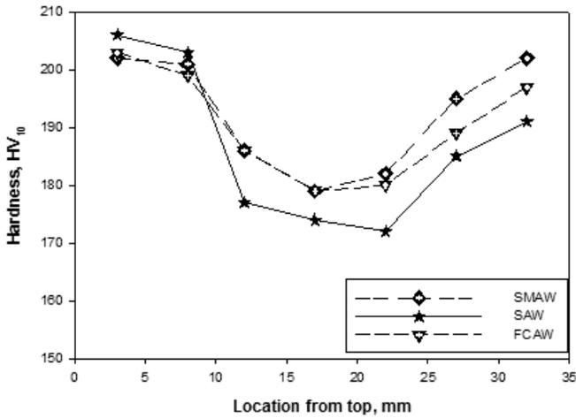
Fig.2. Hardness at different location
