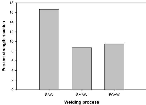
Fig.3.d. Strength reduction for different welding process
