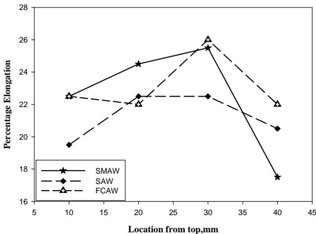
Fig.5. Percentage elongation for different welding process
