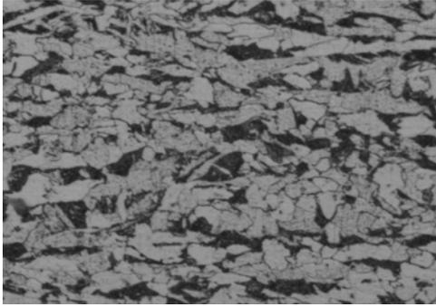
Fig.8.e. Micro structure of base metal
