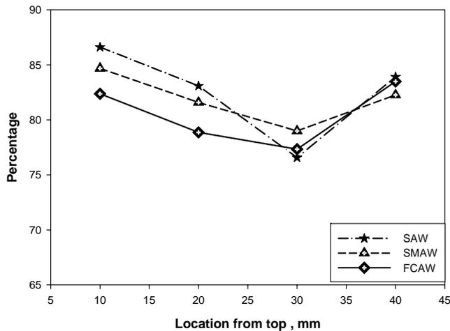
Fig.4. Yield ratio for different welding process
