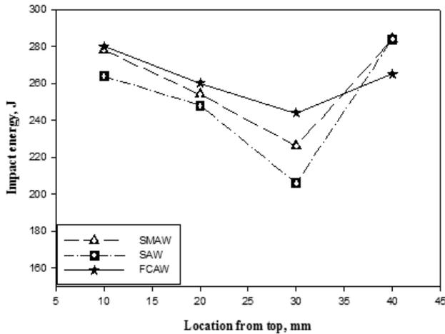
Fig.7. Impact energy at different location
