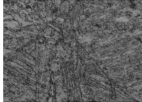
Fig.8.a.Fine grain martensite structure @HAZ
