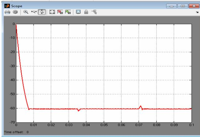
Figure 5 Closed loop response of Triple-Lift Luo converter with sudden disturbances of 3.5msec & 7msec  $\pm$  20% of rated Load
