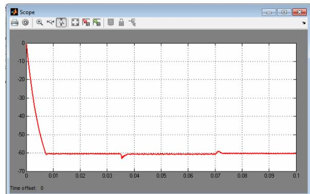
Figure 4 Closed loop response of Triple-Lift Luo converter with sudden disturbances of at 3.5msec & 7msec  $\pm 25\%$  of rated supply
