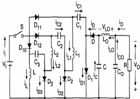
Figure 1 Negative Output Triple-Lift Luo converter
