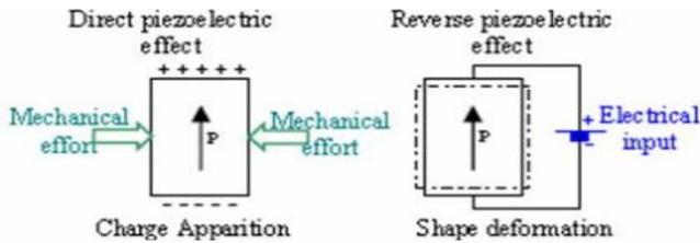
Fig.2: Electromechanical conversion via piezoelectricity phenomenon.
