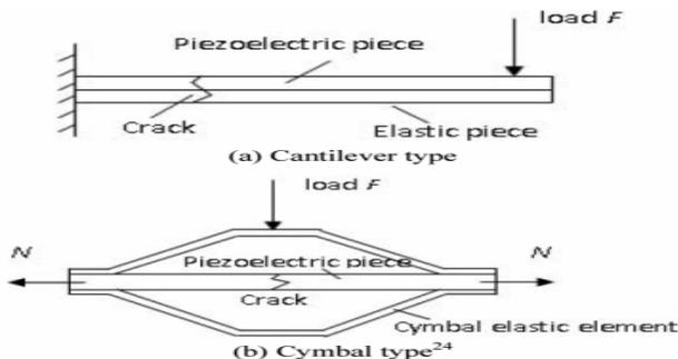
Fig. 4 Conventional piezoelectric energy harvesters
