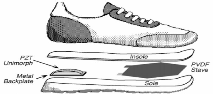
Fig.10: Shoes with Piezoelectric material.
