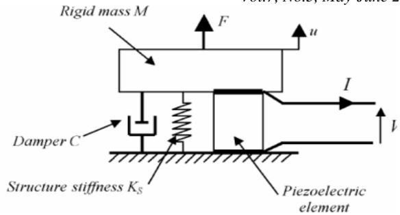
Fig. 5 Model of a vibrating structure including a piezoelectric element [23]
