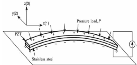
Fig. 6 Curved PZT unimorph excited in d31-mode by a normal distributed force [24]
