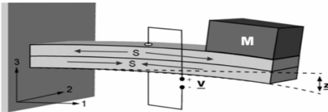
Fig. 3 A two-layer bender mounted as a cantilever (a) Cantilever type (b) Cymbal type[24]
