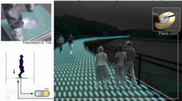
Fig.9: Pathways with Piezo material generating electricity. The energy generated from the moving vehicles is stored in huge batteries and from the batteries the energy is used for the city's energy consumption. This can be used for example to light the street lights at night from the entire energy stored in the batteries. It can also be used for powering the household gadgets and in short the city as a whole saving lots of fuel used in electricity generation in an eco-friendly way.
