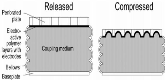
Figure 7. Schematic view of electroactive polymer heel energy harvester module developed by SRI Intl. (sketch based on [29]).
