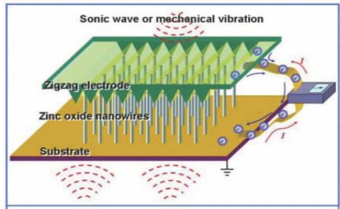
Figure 8 Schematic diagram showing the DC nanogenerator built using aligned ZnO nanowire arrays with a zigzag top electrode.[37]
