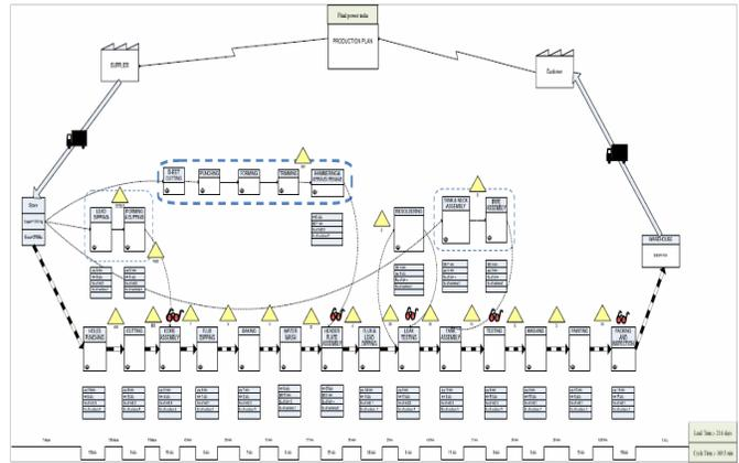
Figure 4. Current value stream mapping
