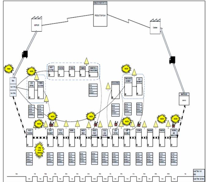
Figure 14. Future state value stream mapping
