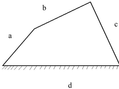
Fig. 2: A simple four bar mechanism
