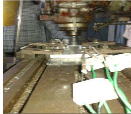
Fig. 4. FSW experimental Set-up
