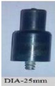
Fig. 3. Fabricated FSW Tool with threaded tip
