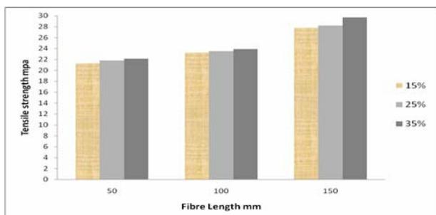
Fig. 5 Effect of fiber parameter on tensile strength
