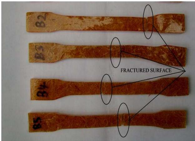
Fig. 4 Photograph of specimens after tensile fracture
