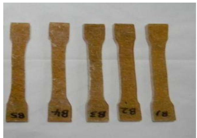
Fig. 3 Photograph of specimens before tensile testing
