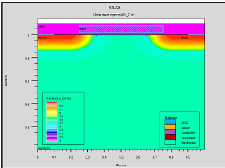
Figure2: The cross sectional structure of Floating Gate MOSFETs using Silvaco TCAD Athena
