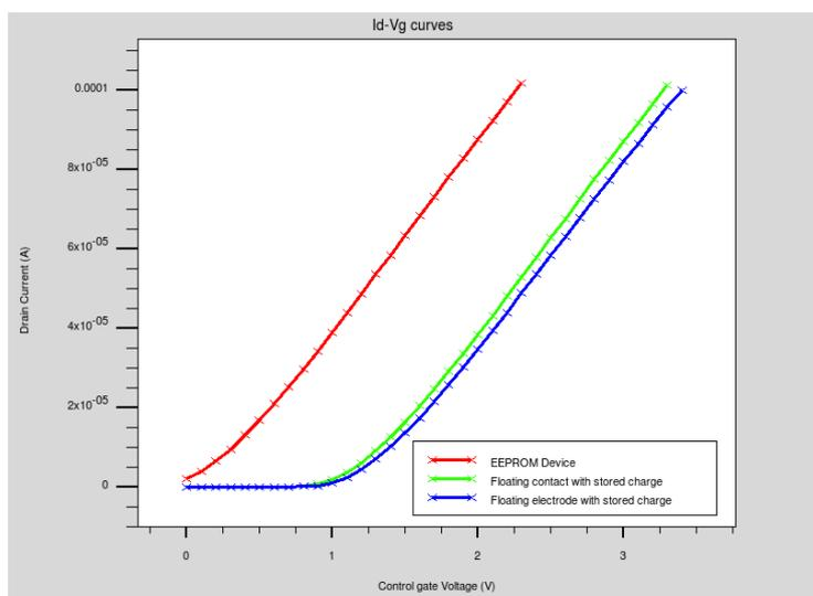
Figure 3: Graph of  $I_{DS}$  Vs  $V_{GS}$
