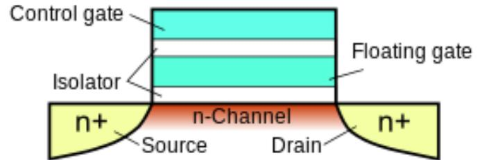
Figure 1: Structure of Floating gate mosfet
