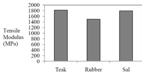
Figure 5. Effect of wood types on tensile modulus of composites
