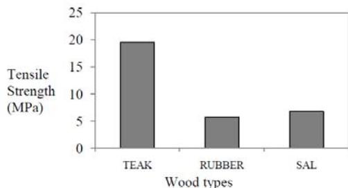
Figure 4. Effect of wood types on tensile strength of composites
