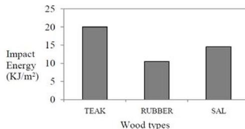
Figure 6. Effect of wood types on impact strength of composites
