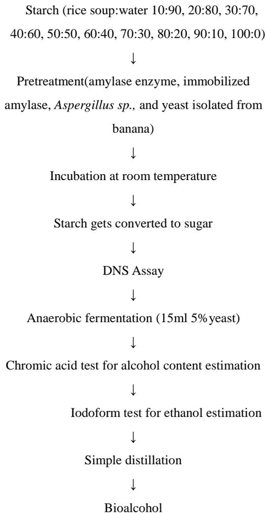
Fig 1: Flow Chart for the preparation of Bioalcohol from rice soup
