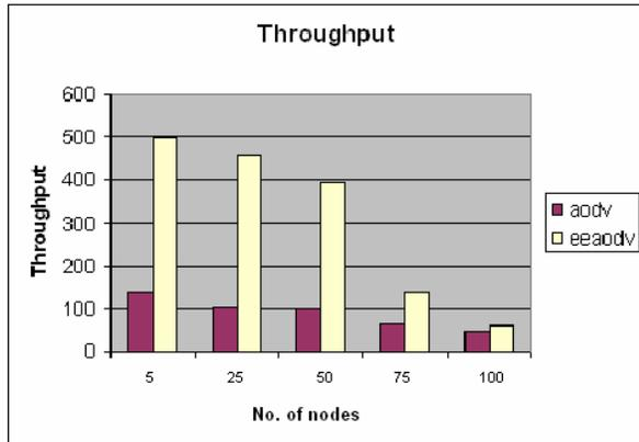
In the scenario performed, eeaodv shows higher throughput (i.e. no. of requests processed) as compared to aodv.
