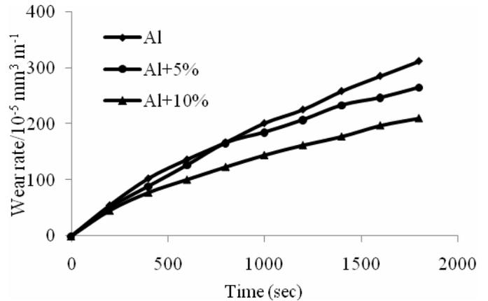
Fig 9. Time Vs Wear rate (rpm = 400 & Load = 5 Kg )
