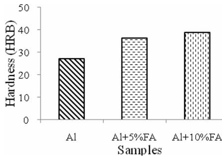
Fig.8 Effect of fly ash on hardness
