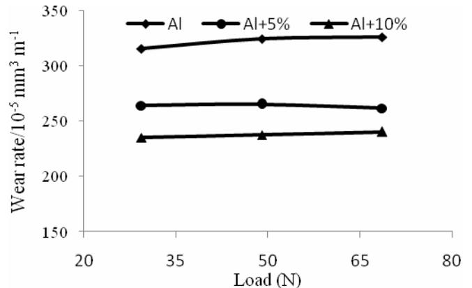
Fig.10 Load Vs Wear rate (rpm = 400 & Time = 1500 sec)
