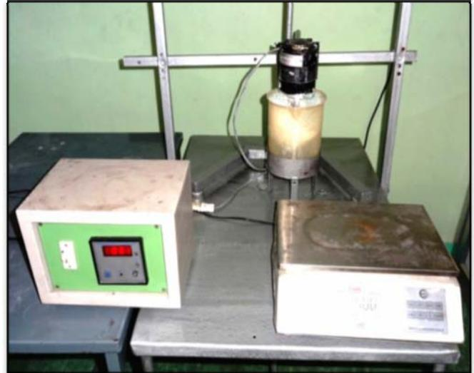
Fig. 5. Wet erosion test setup
