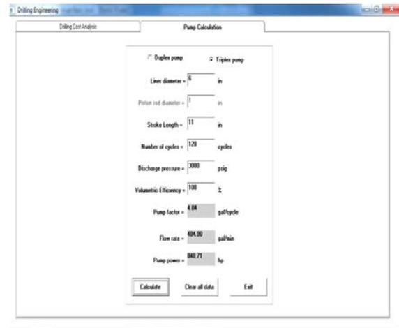
Figure 4: Canned program developed to calculate pump power and efficiency of pump
