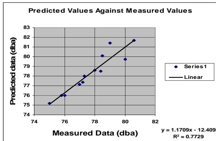
Fig. 2: Relationship Between Measured and Predicted Noise Levels.
