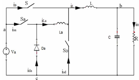
Figure 1. Proposed four switch buck converter
