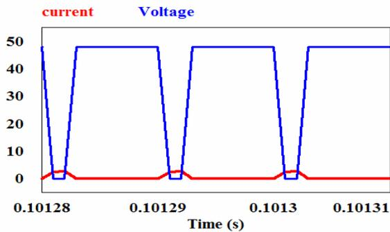
Figure 8. Switching loss across outer cell switch
