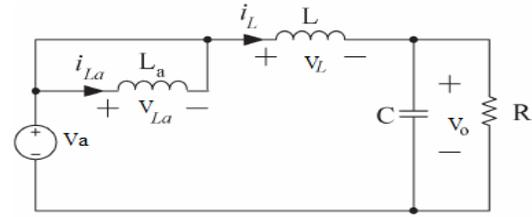
Figure 3. Equivalent circuit of four switch buck converter when  $S=ON, S_a=ON$ .
