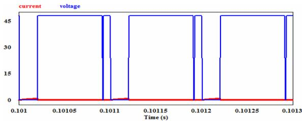
Figure 9. Switching loss across inner cell switch
