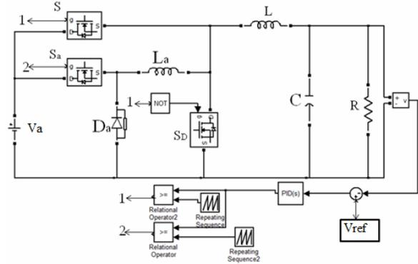
Figure 7. Four switch buck converter with PID controller
