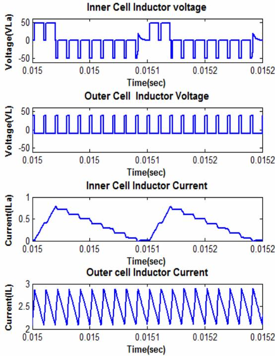
Figure 2. Voltage and current waveforms in switching period  $T_{si}$ .
