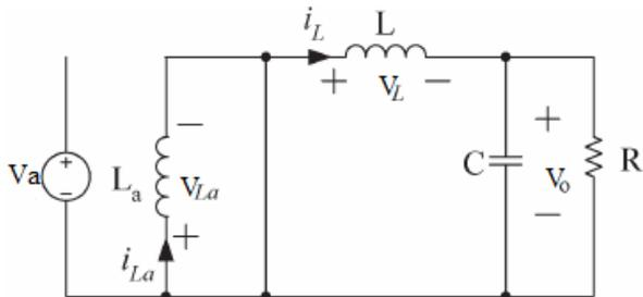
Figure 6. Equivalent circuit of four switch buck converter when S=OFF, Sa=OFF.
