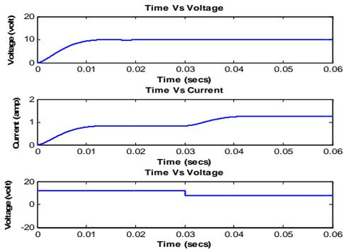
Figure 15. Simulation result of four switch buck converter with load side disturbance
