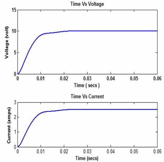
Figure 14. Simulation result of four switch buck converter
