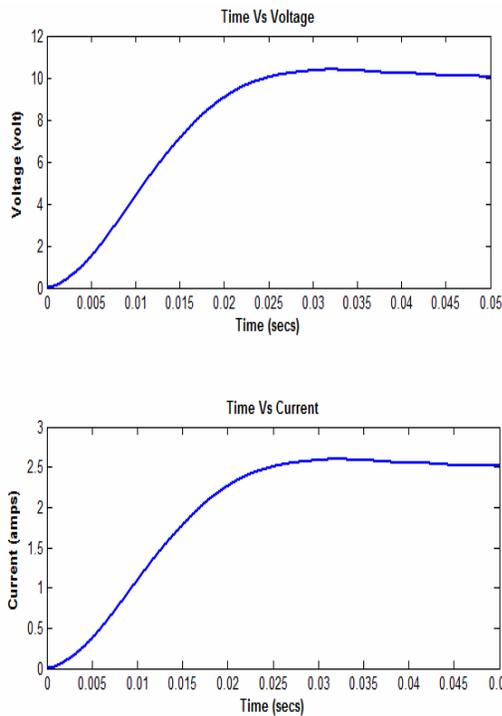
Figure 13. Simulation result of high frequency buck converter
