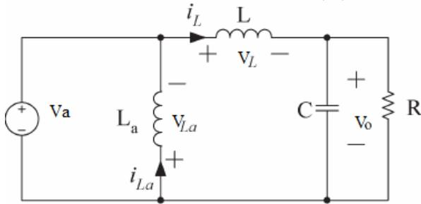
Figure 5. Equivalent circuit of four switch buck converter when S=ON, Sa=OFF.
