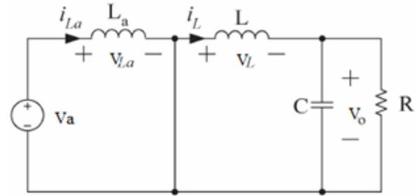
Figure 4. Equivalent circuit of four switch buck converter when  $S=OFF, S_a=ON$ .
