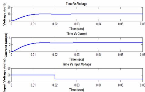
Figure 16. Simulation result of four switch buck converter with source side disturbance
