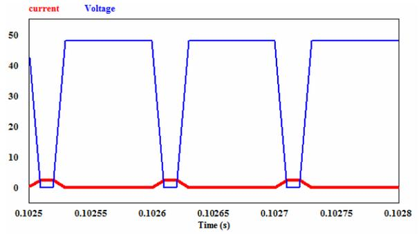
Figure 11. Switching loss of Single Low frequency converter
