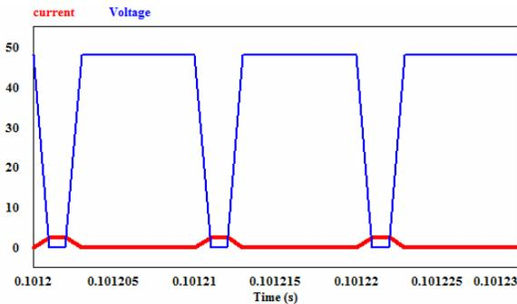
Figure 10. Switching loss of Single High frequency converter
