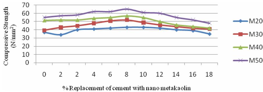
Figure 7: Compressive strength of Concrete at 56th day for Various Replacement percentages of nano Metakaolin.
