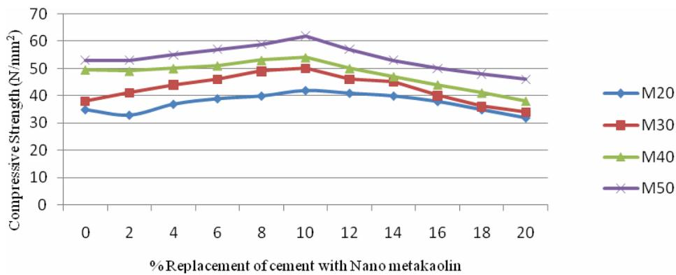
Figure 5: Compressive strength of Concrete at 35th day for Various Replacement percentages of nano Metakaolin.
