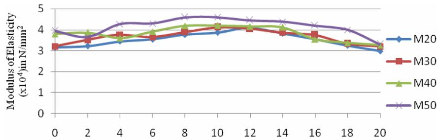
Figure 11: Modulus of Elasticity of Concrete at 56th day for Various Replacement percentages of nano Metakaolin.
