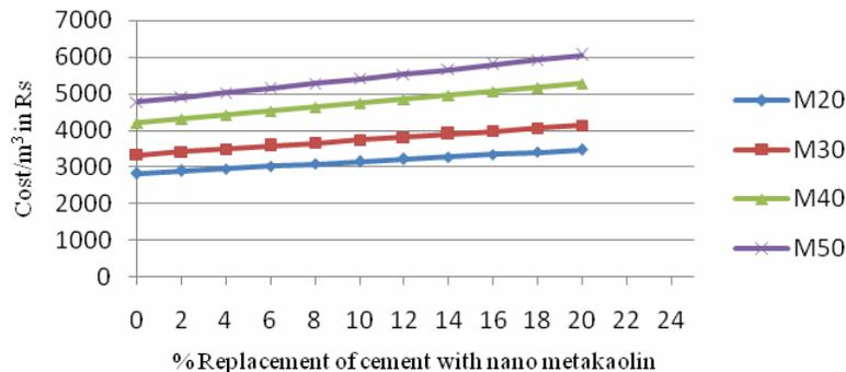
Figure 12: Comparison of Cost of 1 m<sup>3</sup> of Concrete in Rs
