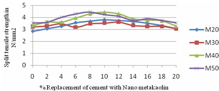
Figure 9: Split Tensile Strength of Concrete at 56th day for Various Replacement percentages of nano Metakaolin.
