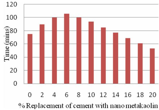
Figure 3: Variation of Initial Setting Time of Cement Paste with Respect to Various Percentages of Nano Metakolin
