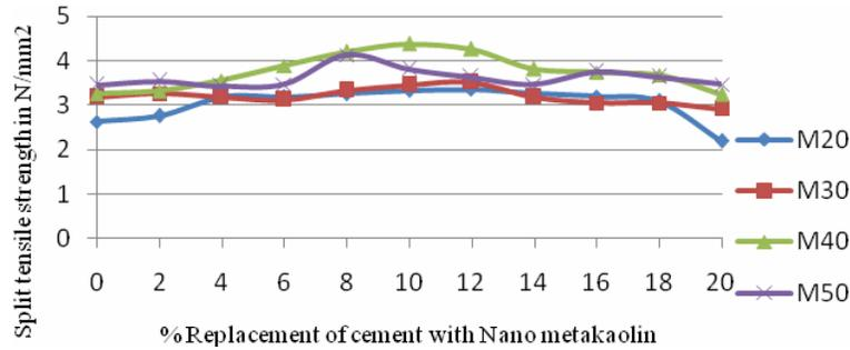
Figure 8: Split Tensile Strength of Concrete at 28th day for Various Replacement percentages of nano Metakaolin.
