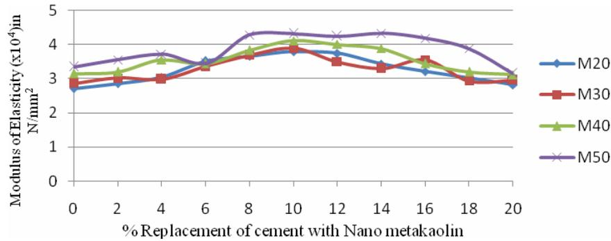
Figure 10: Modulus of Elasticity of Concrete at 28th day for Various Replacement percentages of nano Metakaolin.
