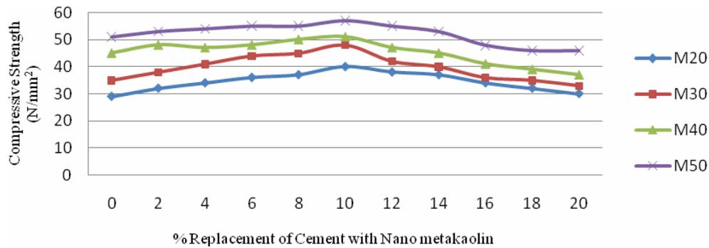
Figure 5: Compressive strength of Concrete at 28th day for Various Replacement percentages of nano Metakaolin.
