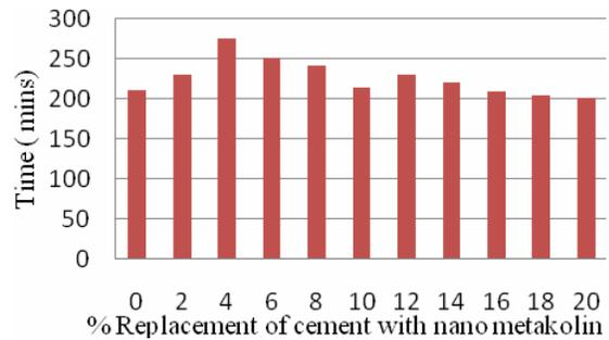
Figure 4: Variation of Final Setting Time of Cement Paste with Respect to Various Percentages of Nano Metakolin
