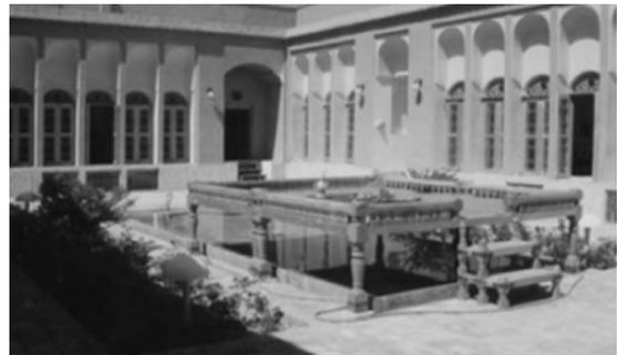
Figure4: Yazd, the central yard and the role of the pond in increasing the humidity
