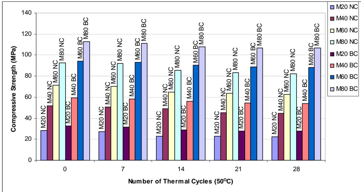
Fig 2: Graph showing Compressive strength of Controlled Concrete and Bacterial Concrete of Different Grades subjected to number of thermal cycles of 50°C temperature
