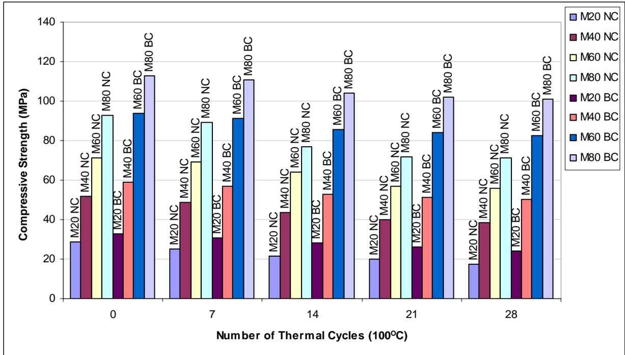
Fig 3: Graph showing Compressive strength of Controlled Concrete and Bacterial Concrete of Different Grades subjected to number of thermal cycles of 100°C temperature
