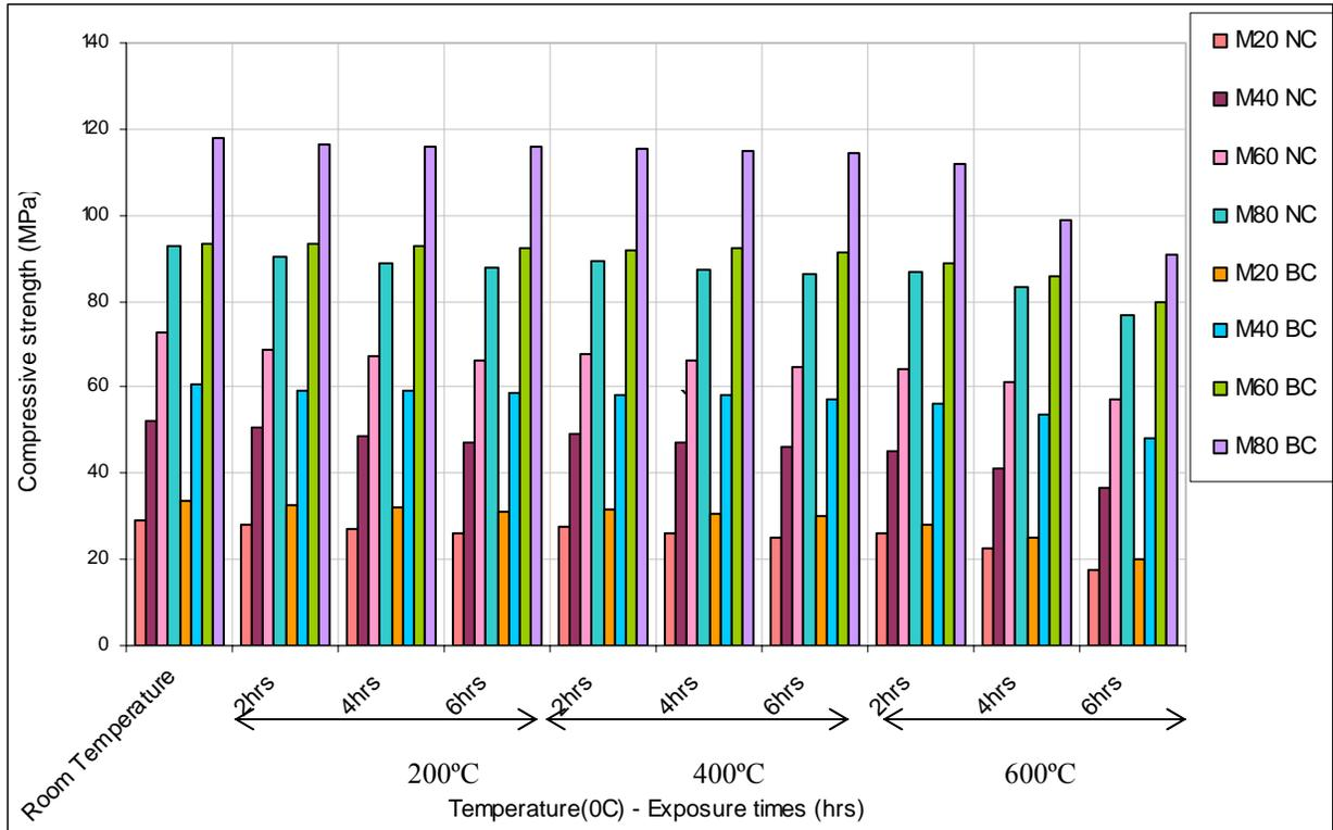
Fig 1: Graph showing variation of compressive strength at various temperatures and exposure durations for different grades of controlled and bacterial concrete
