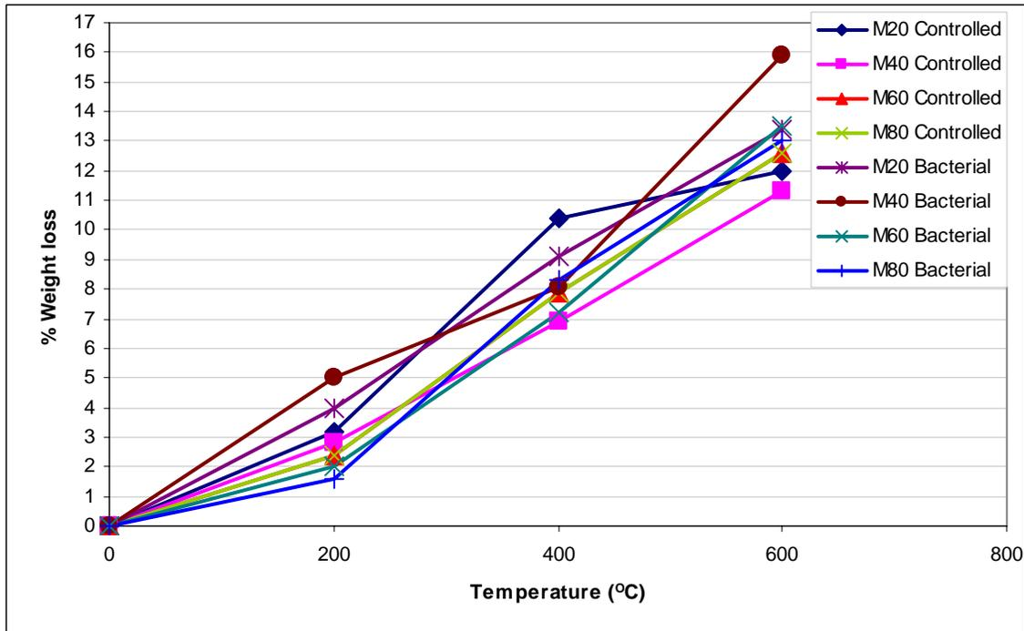
Fig4: Graph showing variation of % Weight Loss at various temperatures for different grades of controlled and bacterial concretes
