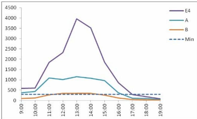
Figure 5. Illumination monitored at points A, B and E4 of the scale models during the day, when the models are orientated due South.
