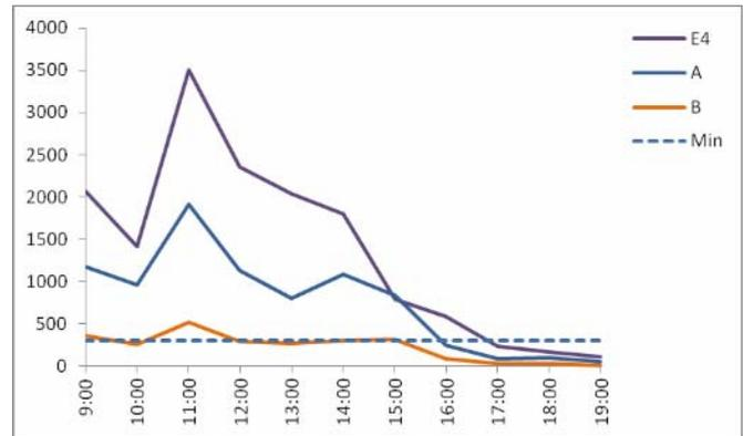
Figure 6. Illumination monitored at points A, B and E4 of the scale models during the day, when the models are orientated due East.
