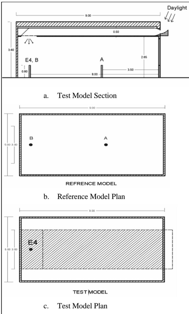
Figure 3. Geometrical configuration of models and the ADS device
