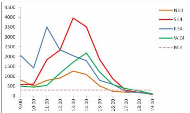
Figure 9. Illumination monitored at points E4 of the test model in four orientations during the day
