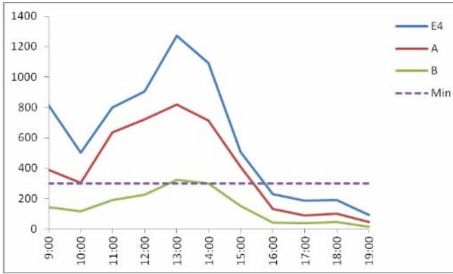
Figure 8. Illumination monitored at points A, B and E4 of the scale models during the day, when the models are orientated due North.
