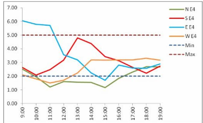
Figure 10. Daylight Factor monitored at points E4 of the test model in four orientations during the day
