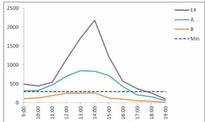
Figure 7. Illumination monitored at points A, B and E4 of the scale models during the day, when the models are orientated due West.
