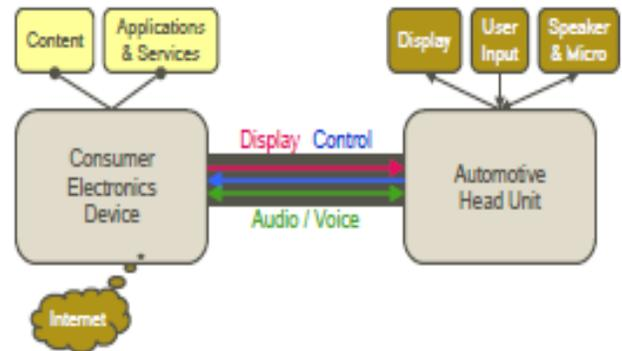
**Figure 1. Terminal Mode Concept**
