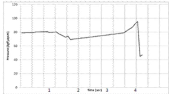
Figure 14. Predicted Pressure – Time Plot for Burning of CMDB Star Shape Propellant
