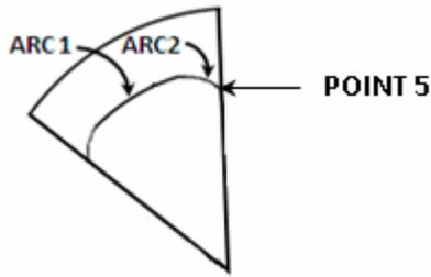
Figure 13. Geometry of Burning Surface Area Phase III
