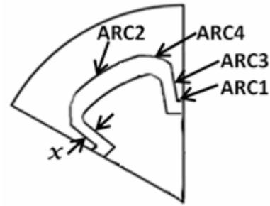
Figure 11. Geometry of Burning Surface Area Phase I
