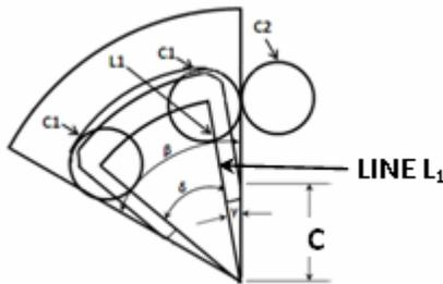
Figure 10. Geometry of Change Over Point Phase II
