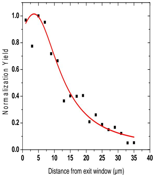
Figure 3: Stopping range of 4MeV  $He^{++}$  ion beam in air.
