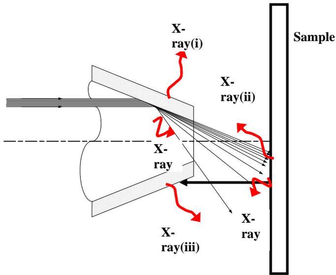
Figure 6: Possibility of Si X-ray generation due to glass capillary itself.
