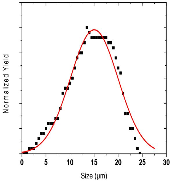
Figure 2: Estimation of beam size produced by 10μm capillary at energy of 4MeV  $He^{++}$ .
