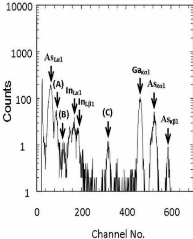
Figure 5: PIXE spectra of GaInNAs sample obtained with a 4 MeV  $\text{He}^{++}$  in-air. The ion beam dose is 1.4  $\mu\text{C}$ .
