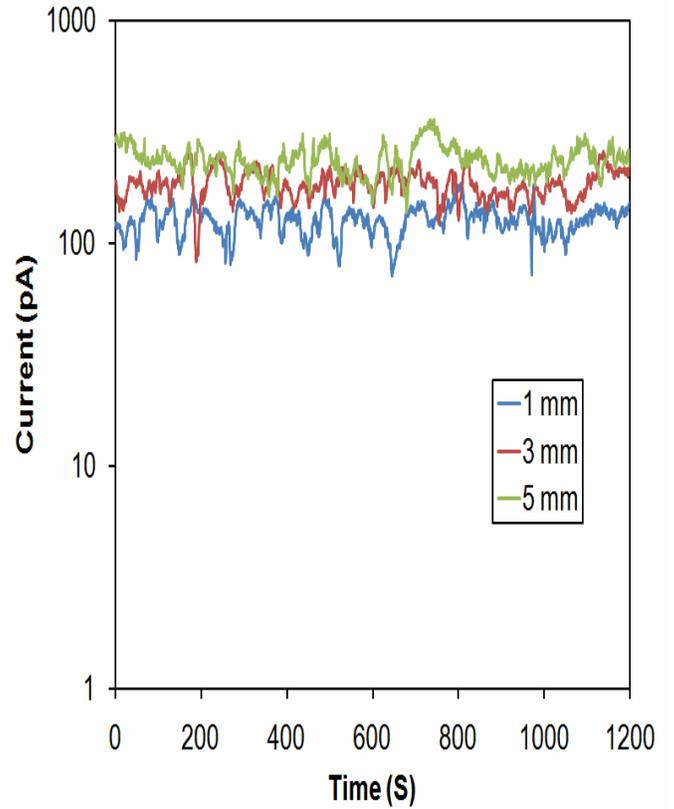
Figure 4: Integrated current with respect of time at different distances from the exit window of the capillary.
