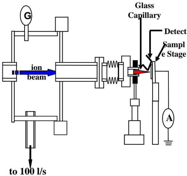
Figure 1: Experimental setup of external microbeam at KUT.
